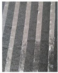
The adhesive coating with lines of adhesive spaced by several mm in width without adhesive, brings a better acoustical effect to panels fitted with it.
